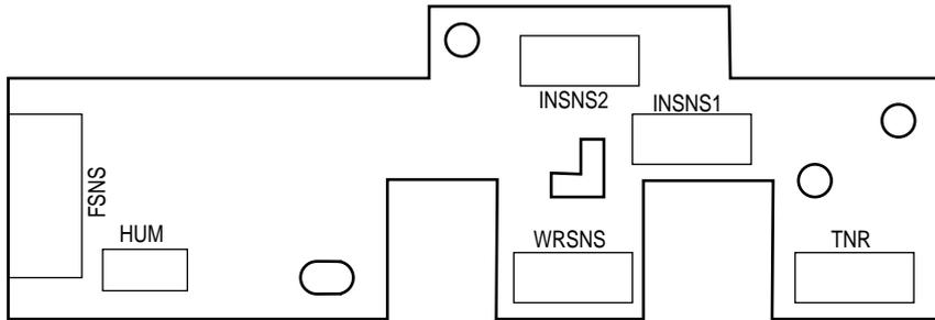
(8) Paper Size Sensing PWB PXC (B73- PWB)
