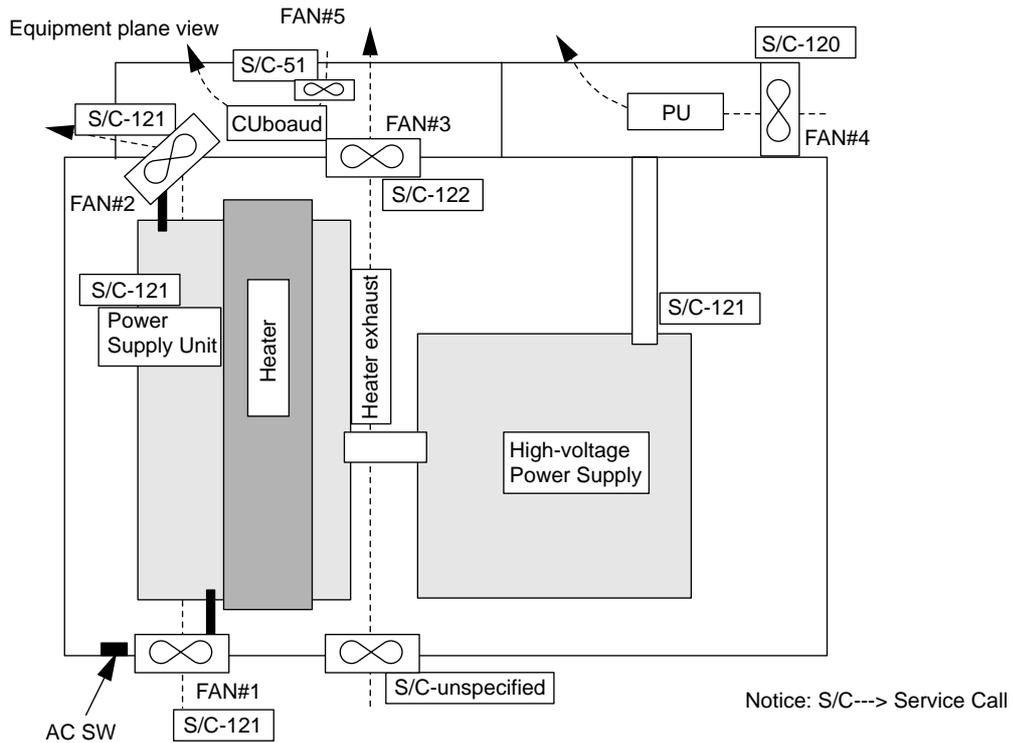
Figure 5.5.1 A Power Supply-related Error
