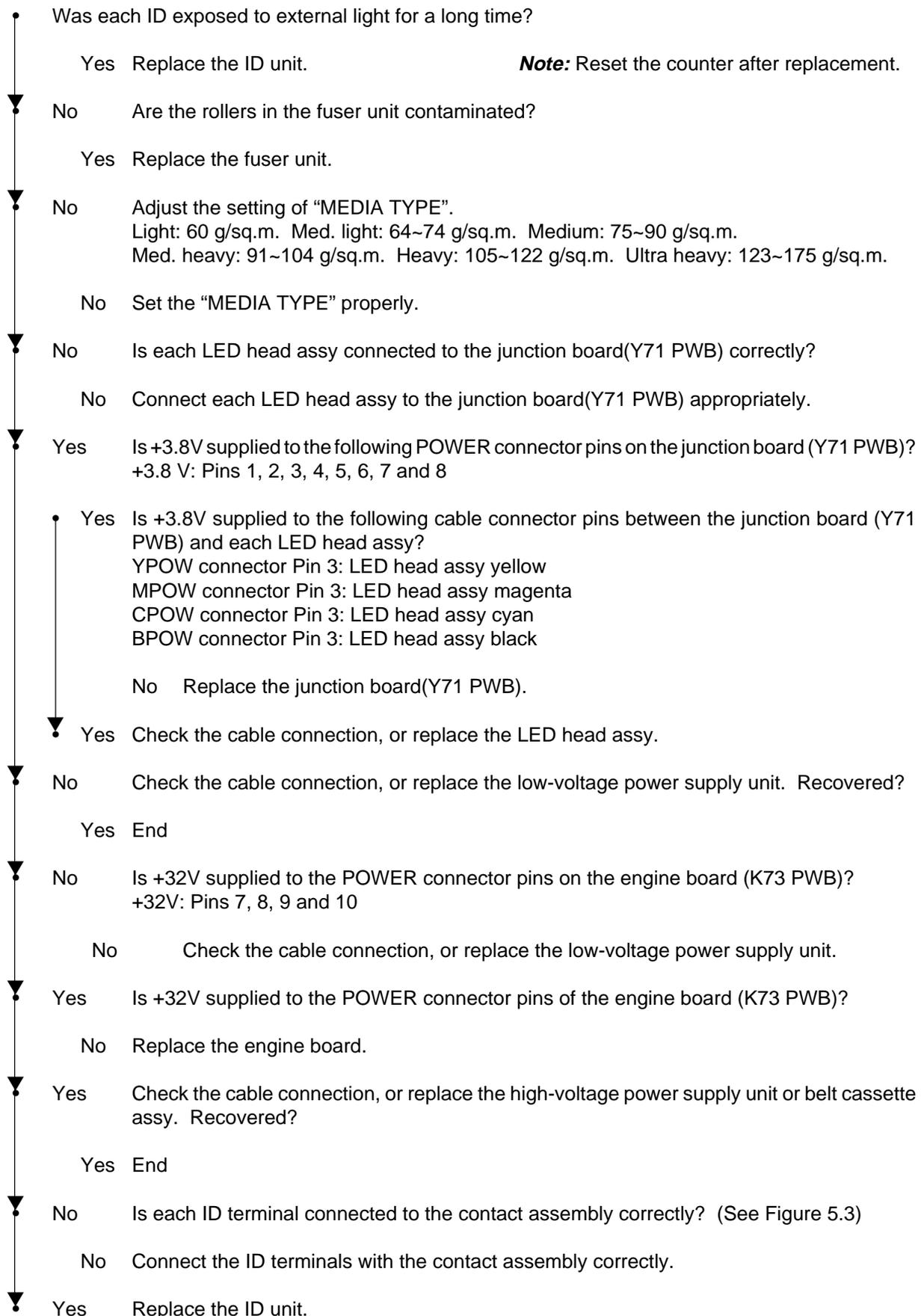
Notes: When replacing the engine board (K73 PWB), demount the EEPROM chip from the old engine board and remount it on the new one.
