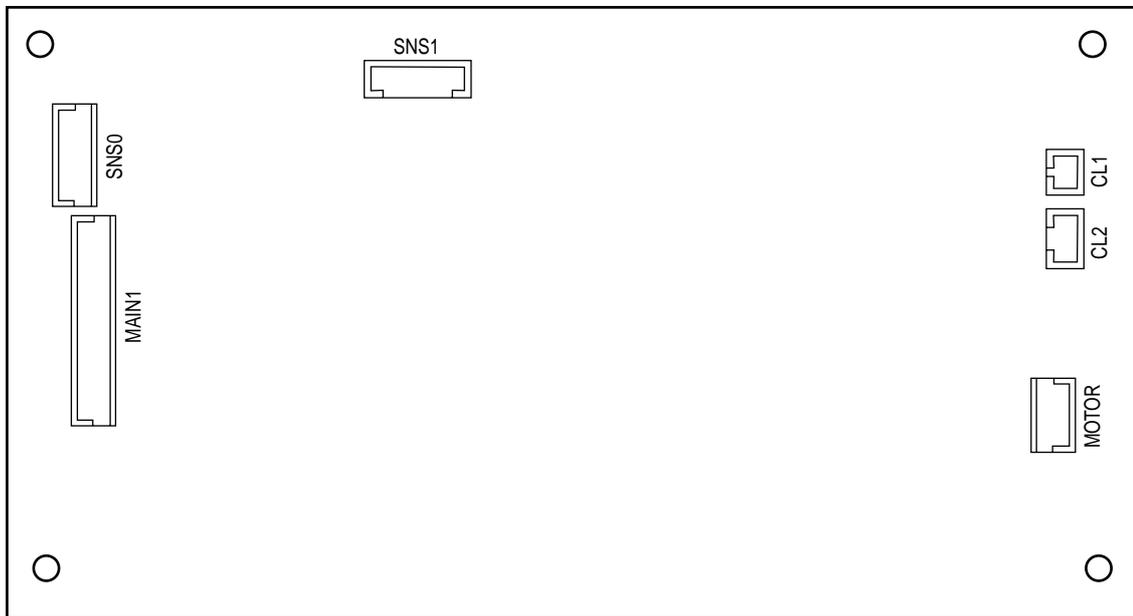
(5) Control Panel PWB (X71- PWB)
