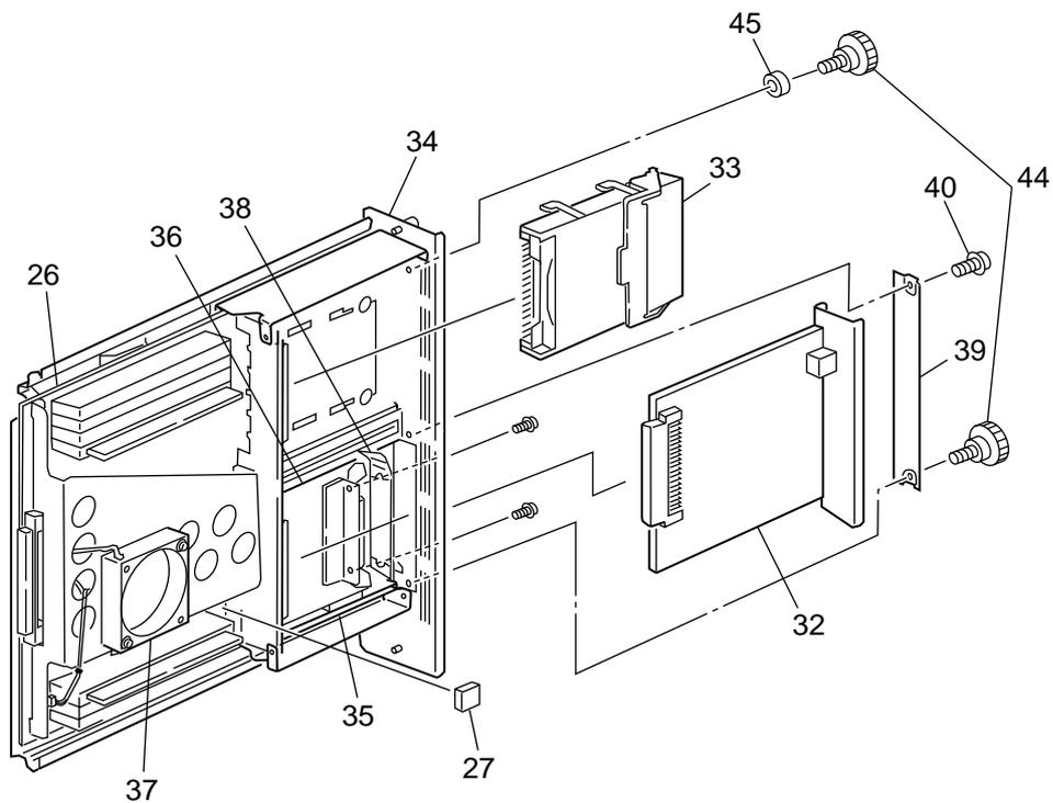
Board Assy.-CU(Maintenance) 34 [41848502] consists of a set of a bracket to support Motor Fan 37 (41410201), a sheet metal to secure PCB Assy-SWA 26 (41716819, 41716820), a gasket bonded to that sheet metal, and screws (attached to the assembly).
