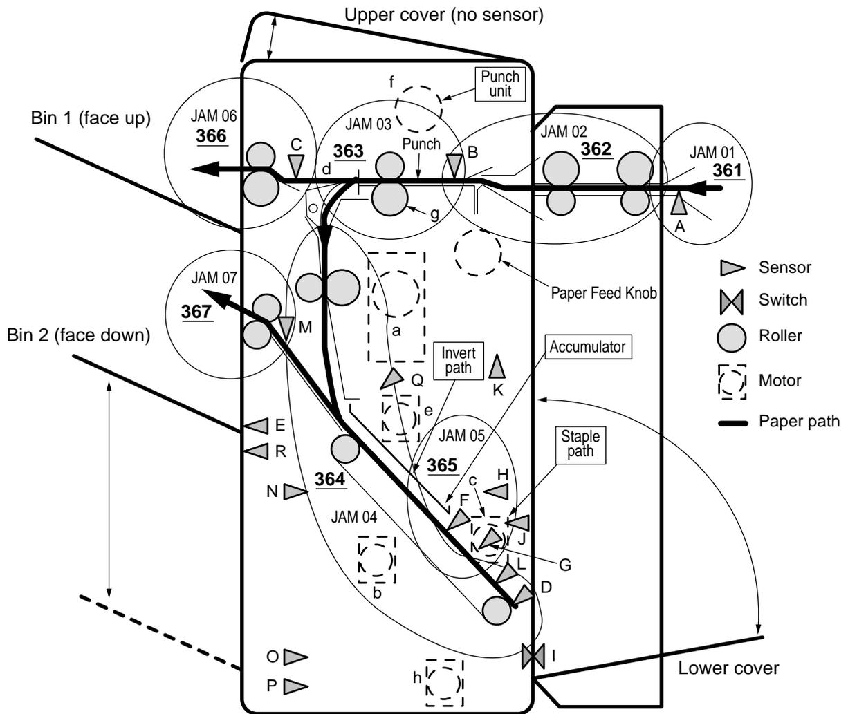
Figure 5.5.2 The position which paper-Jam occurs
